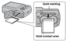
Align the gold marking with the gold contact area, then insert an SD Memory Card completely.
